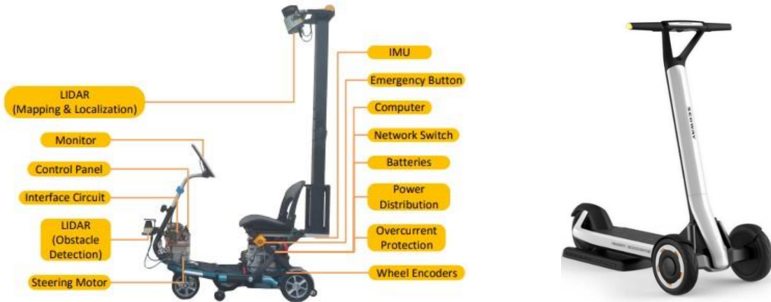
Figure 2.37: Mobility on Demand – Autonomous Personal Mobility Scooter by MIT (left), Self-Driving scooter (right) (Andersen et al., 2016)
