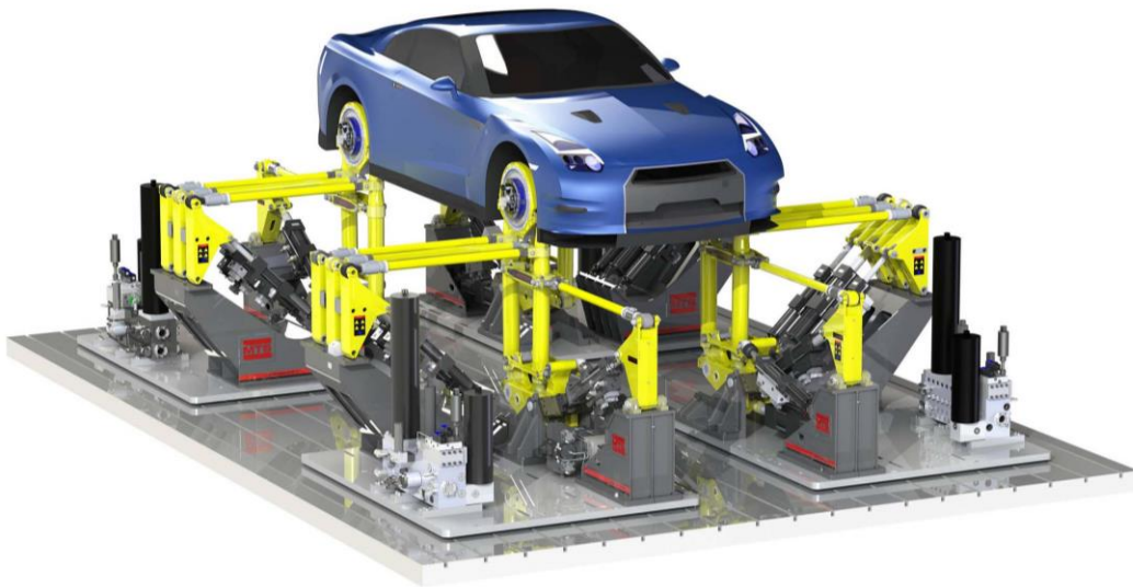
Figure 4.5: Road Simulator Test Rig Used for Vehicle Durability Testing (Source: MTS Systems)
