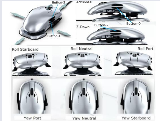
Fig. 4: Essential attributes: The mapping of the WING to the rotational orientations with three degrees—roll ( \Phi ), pitch ( \Theta ) and yaw ( \Psi ) channels.
