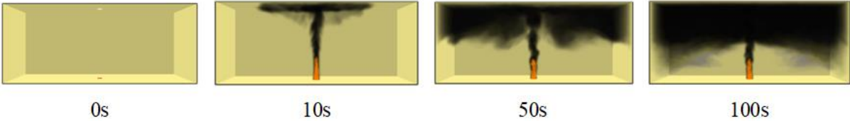
Figure 4-17 Descent of smoke layer height in FDS simulation case FDS-5MW-L50W20H20: 50m Flat Atrium with 20m Width x 20m Height atrium, (5MW) at 0s, 10s, 50s and 100s
