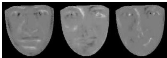
Figure 2.4 Learned appearance variation from the AAM model, adapted with Cootes et al. (2001)
