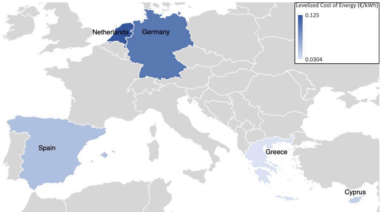
Fig. 5. Heat map of LCOE of 200 kWp PV systems deployment in Northern and Southern European Countries.
