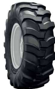
Figure 17. R4 Wide lug tyre (Goodyear)
