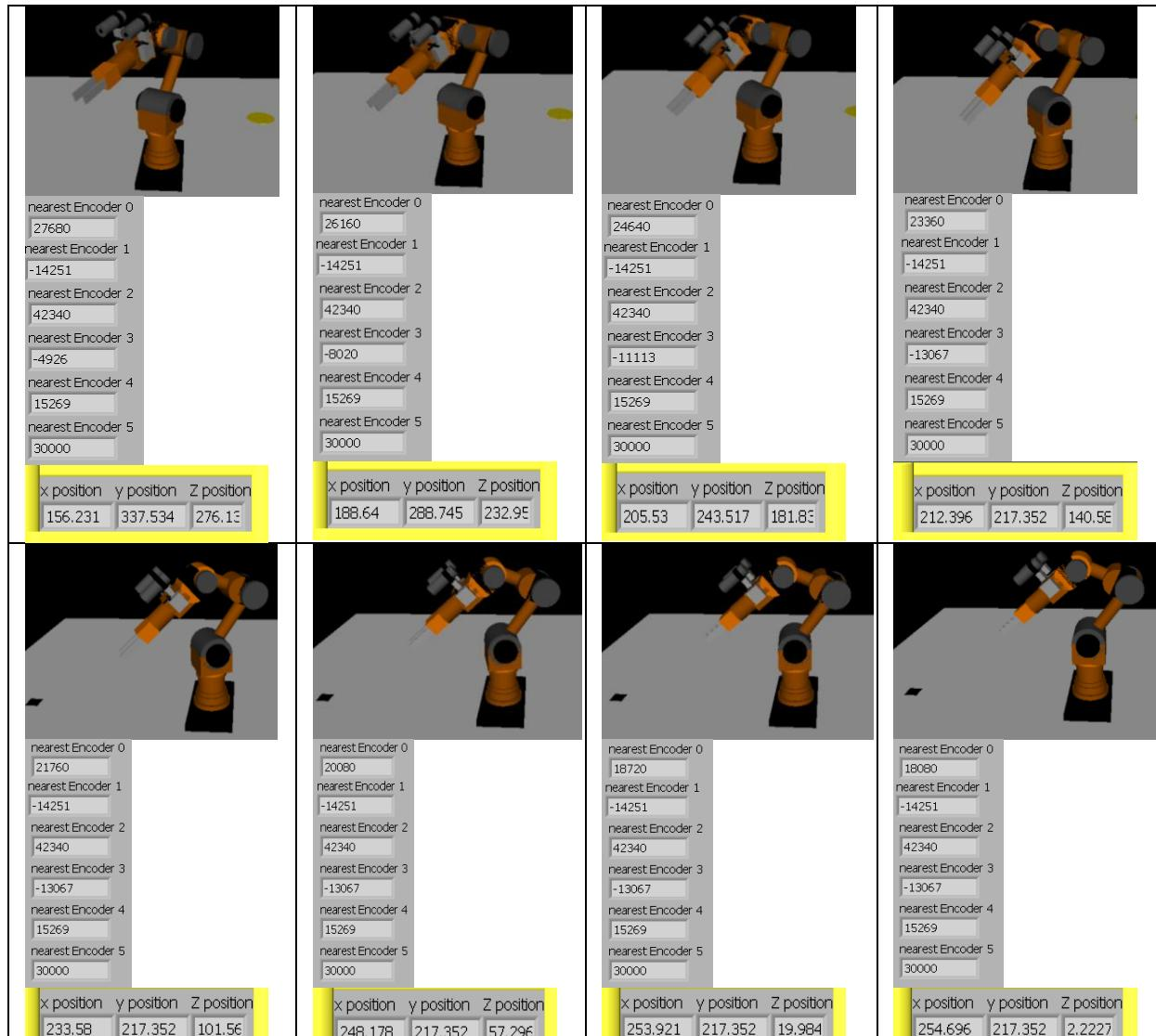
Due to the difference in joint space, the manipulator returns to the first scan position slightly different than the GBOPO ‘drop-off’ point. Although the rotation of Joint 0 is identical the manipulator orientation reaches its final position sooner, therefore the manipulator waits until the rest of the robot arm has completed the revolution to the first scan position.
