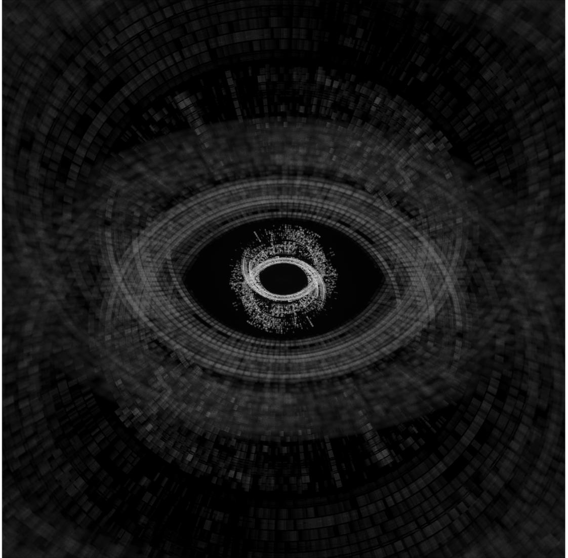
**Figure 6.2:** The e-MERLIN spatial frequency coverage when observing the Lockman Hole, obtained by fourier transforming the CLEANed sky image. There are two noticeable gaps in the coverage at the very centre, and slightly out from the centre.
