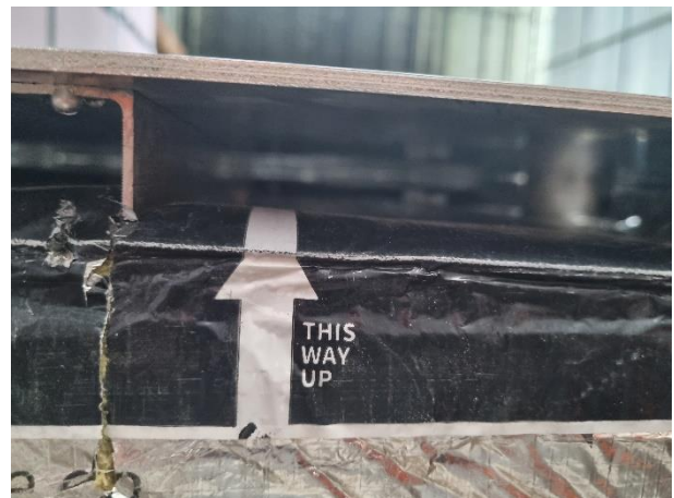
Figure 63 - Photograph of cavity extending from burn chamber opening to top of test rig
