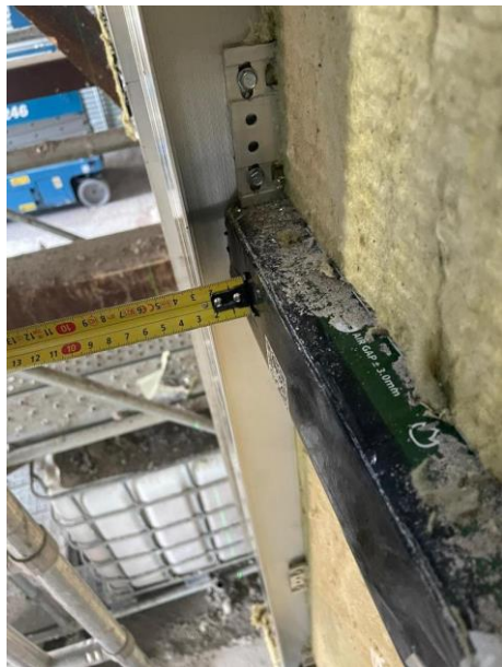
Figure 62 - Open state cavity barrier installed on horizontal edge of burn chamber
