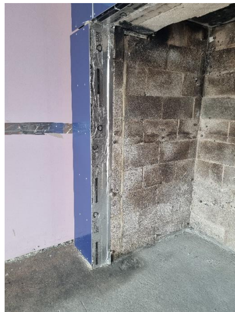
Figure 63 - Photograph of cavity extending from burn chamber opening to top of test rig
