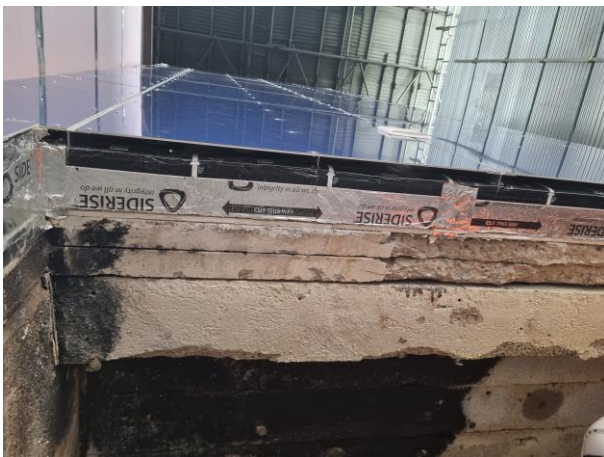
Figure 62 - Open state cavity barrier installed on horizontal edge of burn chamber
