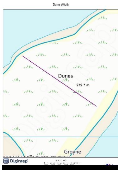
Fig. 8. Dune Width measurement on OS Digimap. Source These pictures were created by the second author using ArcGIS 10.3.1 version on the university's (University College London-UCL) licensed version of ordnance survey and Digimap.
