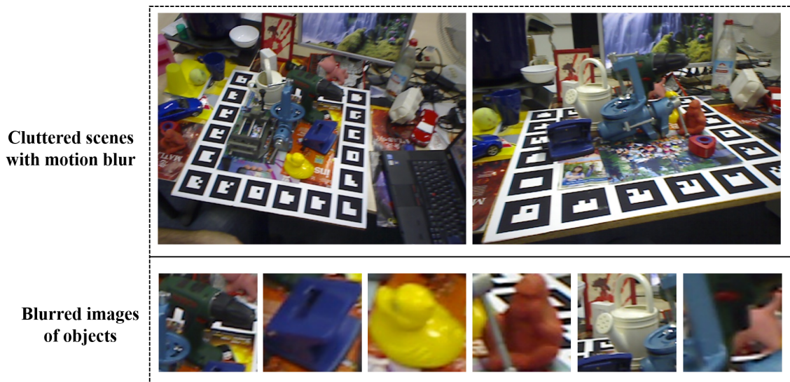
Figure 1.4: Examples of clutter and motion blur. The example scene images depict scenarios with cluttered backgrounds and motion blur that add visual complexity. Simultaneously, the objects of interest demonstrate challenging cases such as occlusion, which complicates the pose estimation task. The images are taken from the Linemod dataset [1, 2].
