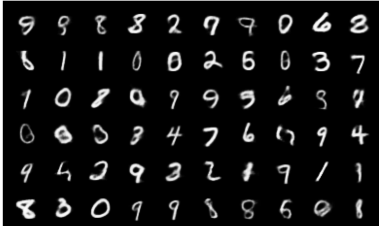
Figure 3.18: Generate new digits from the Gaussian prior using a variational autoencoder. During training, the model is trained to learn both the features and distribution of the MNIST digits dataset [163, 164]. During inference, the encoder network can be discarded and the decoder network can be treated as a generator to create new data from the prior p(z) = \mathcal{N}(z; 0, I) .
