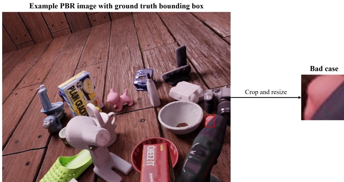
Figure 3.10: Example bad case for the training data. The object visibility information is provided by the Linemod PBR dataset, which is defined as the proportion of the number of visible pixels of the object. The images are taken from the Linemod PBR dataset [1, 2, 7, 8].
