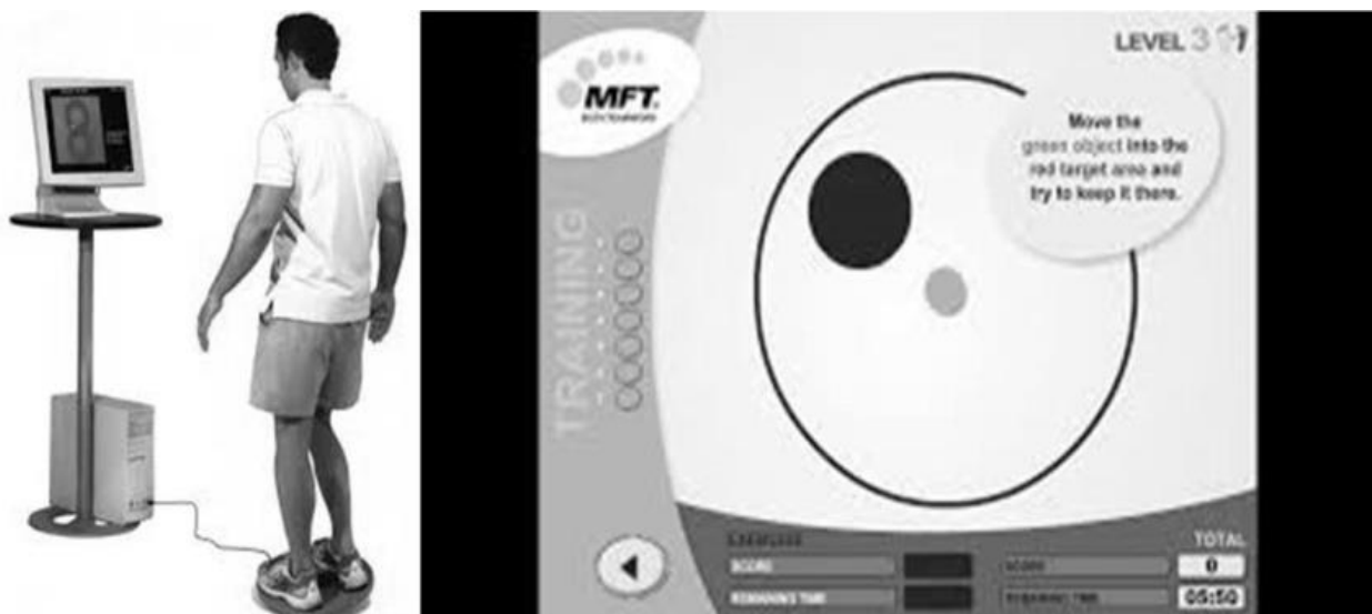
Figure 9: Positioning of the participant on the MFT Challenge disc (left). Screen showing the small dot which should be moved by the participant in the big (darker) dot by shifting the weight on the board (right).
