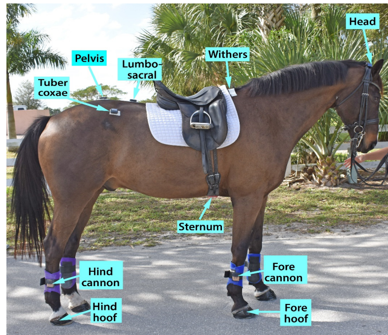
Figure 1. IMU locations. Sensors on the limbs are attached bilaterally. Photo courtesy of Dr. Hilary M. Clayton.
