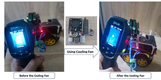
(b) Raspberry Pi before and after the cooling fan.
