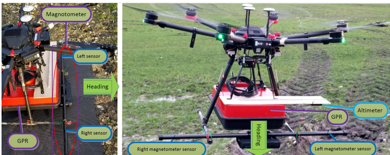
Figure 1: Onboard sensors: Integrated magnetometer and GPR.
