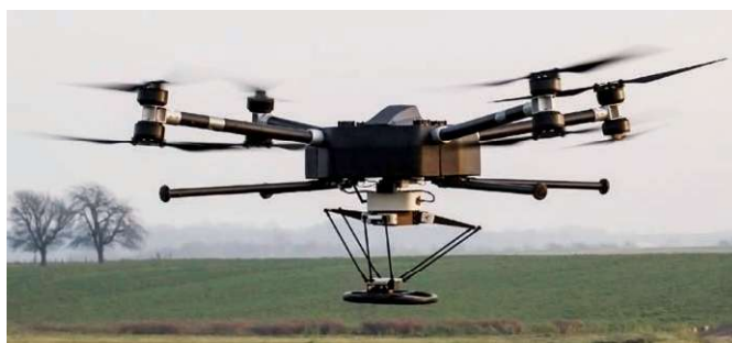
FIGURE 1. MANTA Mine Kafon 1 : GPR and metal detectors.
