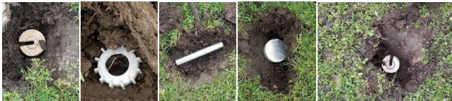
FIGURE 9. Examples for the plastic and metal landmines in different depths in the UCLan landmine field (Fig. 8).
