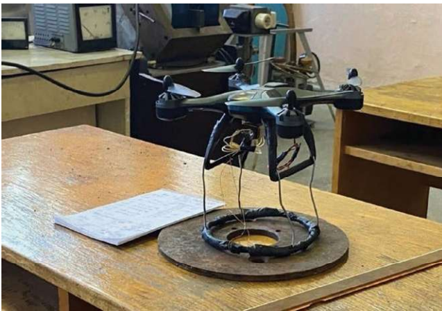
FIGURE 4. F5 PRO quadcopter 4 : invested by NATO, 20–30 mins flight time, no real-time data processing.
