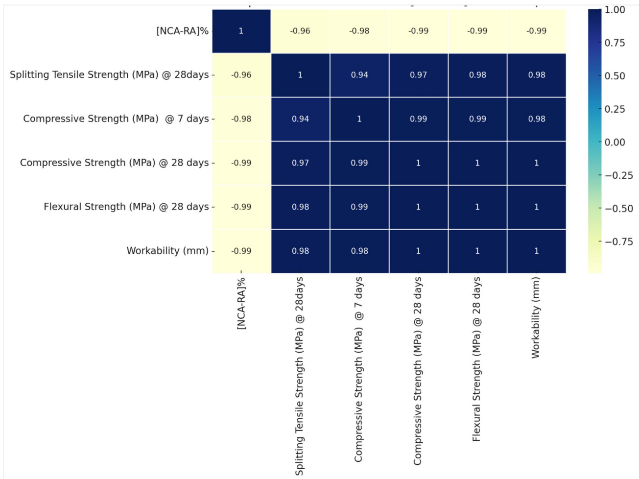
Fig. 5 Correlation Analysis of Concrete Properties and [NCA-RA]%
