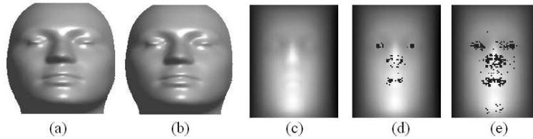
Figure 1: Results for B-spline surface fitting: (a) rendered 3-D data, (b) Fitted B-spline Surface, (c)-(e) display the closest distance maps which respectively are not bigger than 0.5, 0.2, and 0.1 mm (bigger the distance the brighter the point)
