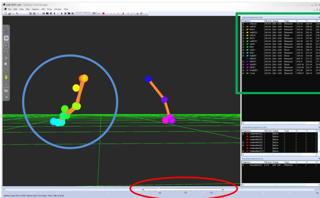
Plate 4.4. Analysis of walk using Qualysis Track Manager™. The limb circled in blue was analysed in the current study. The time line along the bottom has been cropped to one stance phase (circled in red). The Box highlighted in green shows the co-ordinates in X, Y and Z of the different markers at any point on the data clip.
