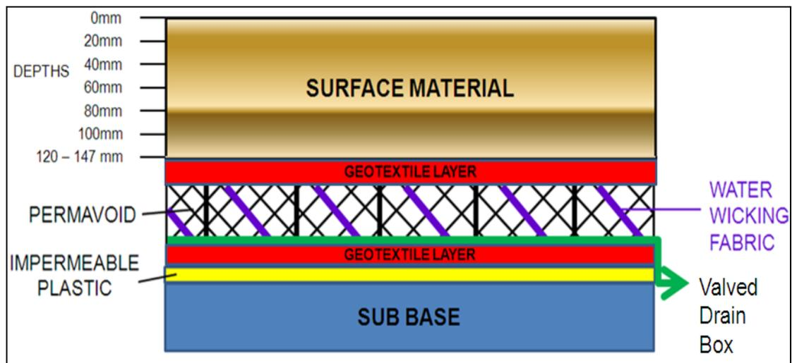
Figure 3.1. Component layers of the test track at Myerscough College. Picture courtesy of Jessica Hawkins, and UCLAN.
