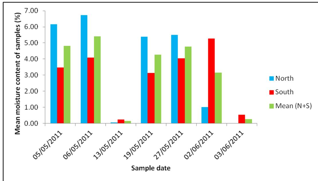
Figure 5.15 Moisture content levels of the surface samples taken from the test track on data collection dates. Samples were taken from the North and South of the track with a mean produced for each (n=3) A mean average (n=6) of the two ends was also produced to give an indication of moisture content of the track as a whole.
