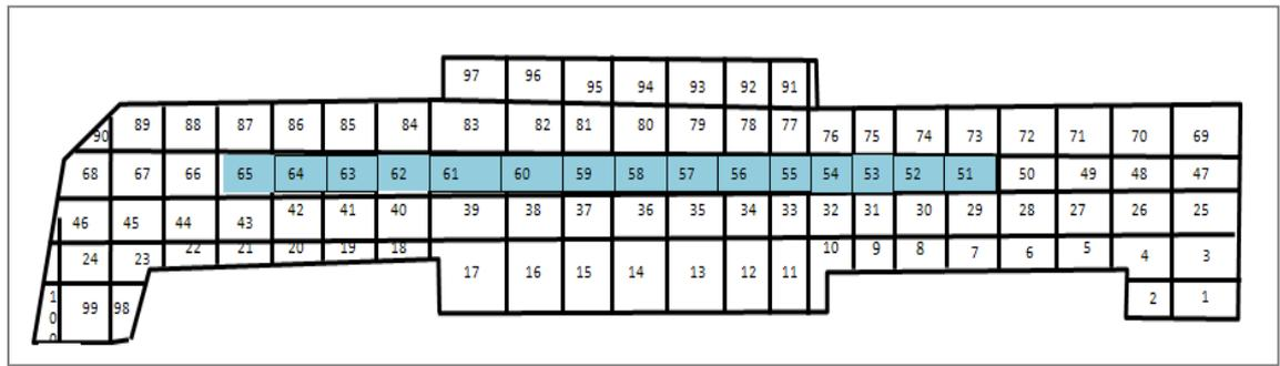
Figure 4.1. Track surface testing grid. Areas 51-65 (shaded in blue) were tested for hardness using a Clegg impact tester after each treatment data collection. The large amount of squares that were not used in the current study were numbered for use in unrelated test work.
