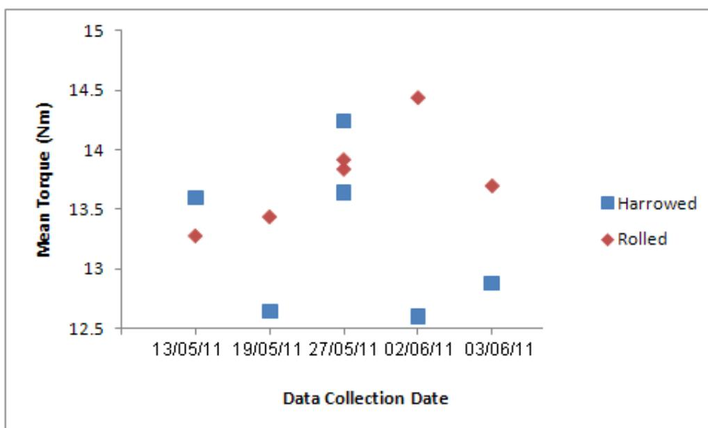
Figure 5.14. Comparison of mean (n=25) surface torque readings (Nm) for treatments (harrowed and rolled) for six out of nine horses on data collection dates, with data for two horses collected on 27/05/11. Data was collected from the smaller selected area for hardness testing (squares 57-61). There was no correlation observed between values ( $p < 0.05$ ).
