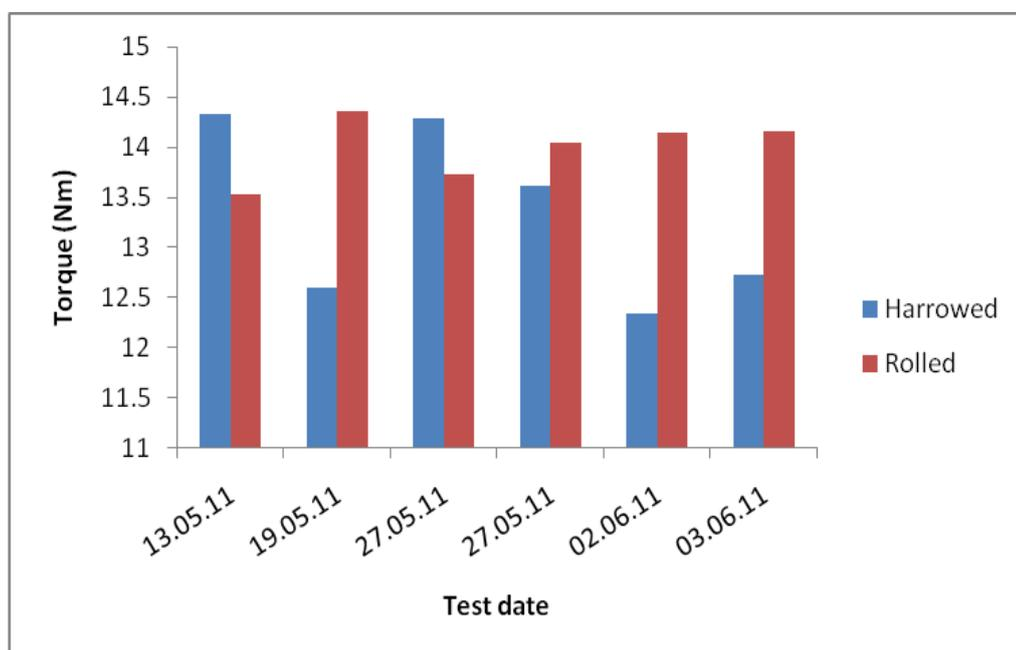
Figure 5.13. Comparison of mean ( $n=75$ ) surface torque readings (Nm) for treatments (harrowed and rolled) for six out of nine horses on data collection days. Data was collected from the originally selected area for hardness testing (squares 51-65). One horse was tested per day, except for the 27/05/11 where two were tested. Data for horses on 27/05/11 is displayed in the order in which it was collected.
