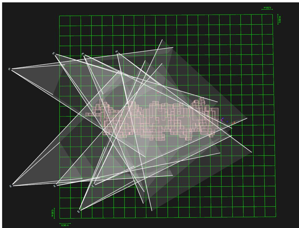
Plate 3.1. Overhead image of the calibrated filming zone used for pilot testing. Overlapping camera fields of view are presented in white. The red cubed volume in the middle represents the calibrated volume that data is collected within. The green grid shows the floor surface area.
