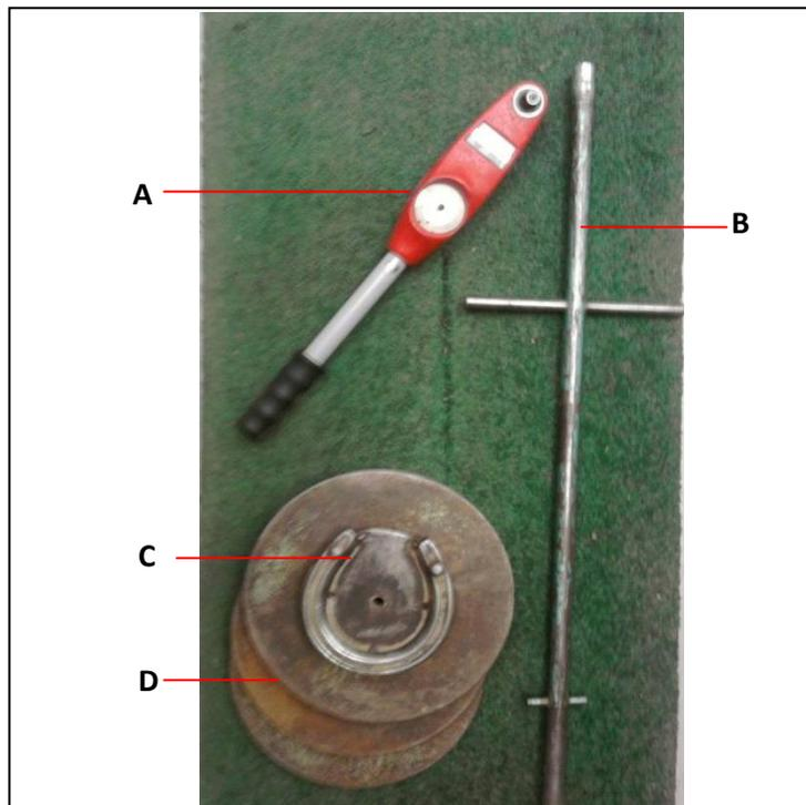
Plate 4.3. Torque wrench split into component parts. A = Torque wrench. B = Connecting section with handles to lift and operate equipment. C = Specially adapted base plate. D = 10Kg weights
