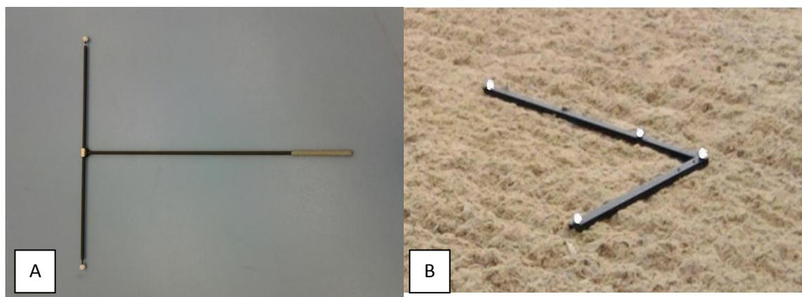
Plate 2.3 Optoelectronic calibration wand with non-coplanar control points (A). The wand must be recorded inside the capture volume for a set time (~60 seconds). Wand motion should be smooth and continuous and cover a 3D volume in all directions and orientations. Optoelectronic calibration L Frame (B) used to establish the orientation of the 3D axis in relation to the camera set up.
