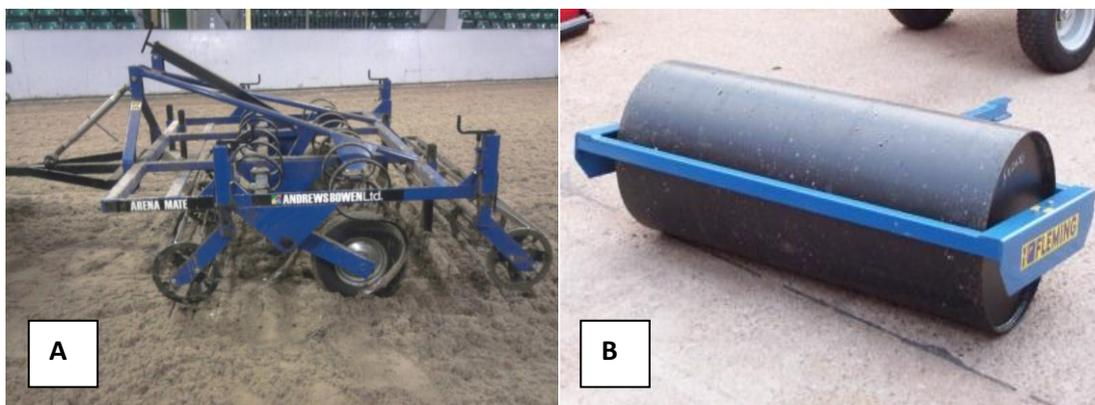
Plate 3.2. A combined harrow and grader (A) comprises of eight tines and two revolving graders. Surface roller (B) used for turf and arena surfaces. Weight of roller = 300 Kg. Width = 2m (landscapemachinery.co.uk).
