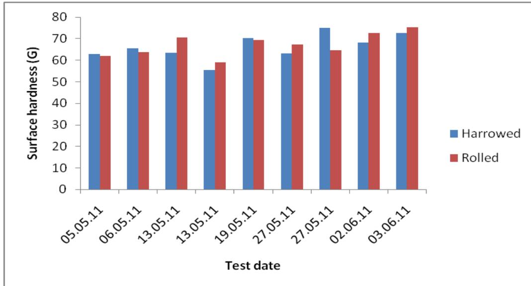
Figure 5.10. Comparison of mean (n=75) surface hardness readings (gravities) for treatments (harrowed and rolled) for each horse on each date of testing. Data was collected from the originally selected area for hardness testing (squares 51-65). One horse was tested on each date, except for the 13<sup>th</sup> and 27<sup>th</sup> May, where two were tested. Data for horses tested on the 13<sup>th</sup> and 27<sup>th</sup> May are displayed in the order in which they were collected.
