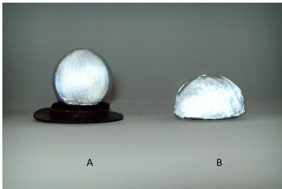
Plate 2.1. Durable, lightweight passive reflective markers. A = Spherical marker (38mm), B = hemispherical (42mm) marker. Markers are foam shapes covered by reflective film (Scotch-lite).
