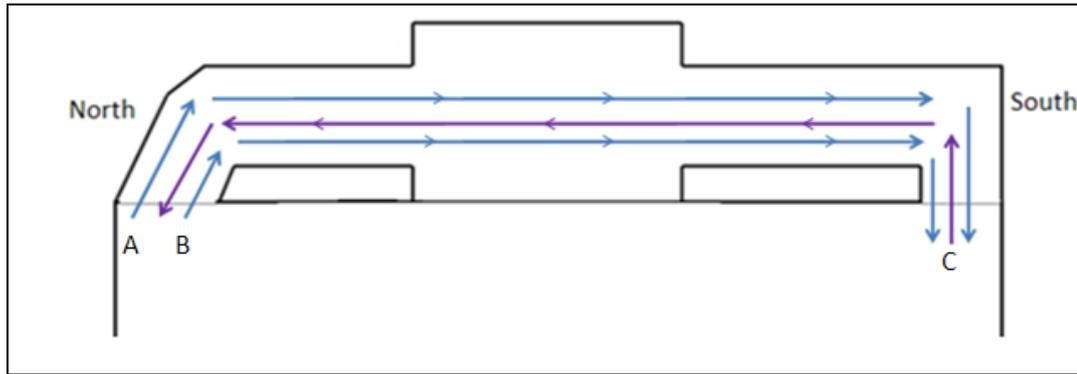
Figure 3.3 Direction of application of arena treatment. A= 1<sup>st</sup> pass North to South; B=2<sup>nd</sup> pass, adjacent to A, North to South; C= 3<sup>rd</sup> pass South to North overlapping the inside area of both A and B.
