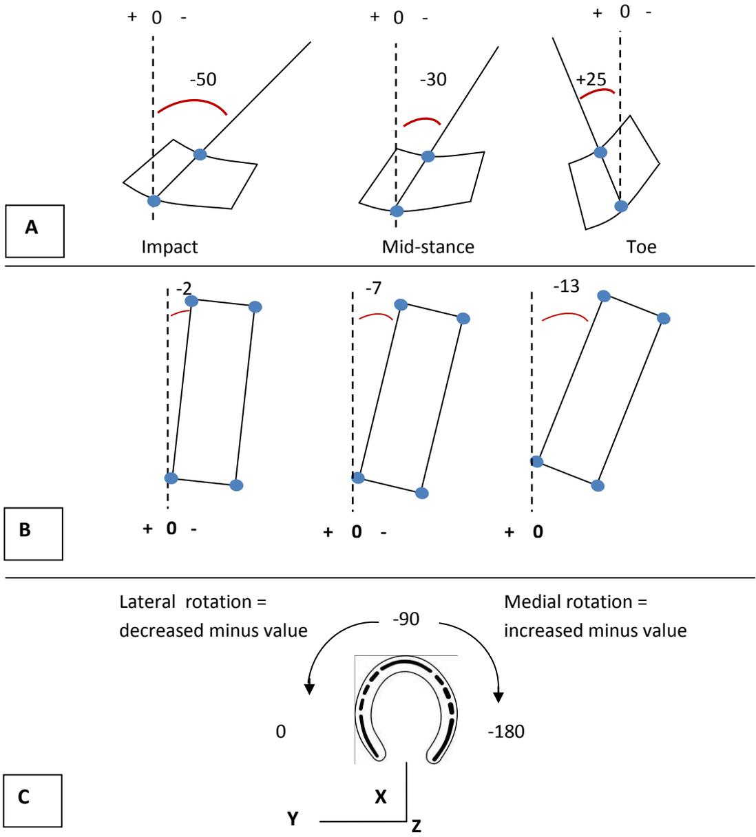
Figure 4.3. Sign conventions for rotation of the hoof and MCIII using the global coordinate system. A) Pitch (forwards/backwards = +/- values), B) Roll (medial/lateral = -/+ values). C) Yaw (lateral/medial= -/+ values).
