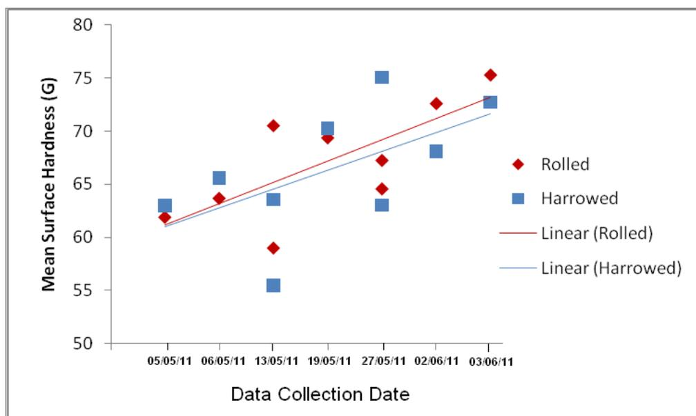
Figure 5.11. A slight trend was observed between mean hardness (n=75) and data collection date for both treatments (harrowed and rolled) on the originally selected area for hardness testing (squares 51-65).
