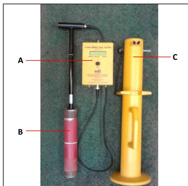
Plate 4.2 Clegg Impact Testing device. A= digital display meter. B= 2.25Kg drop weight fitted with accelerometer. C= Hollow guide tube.
