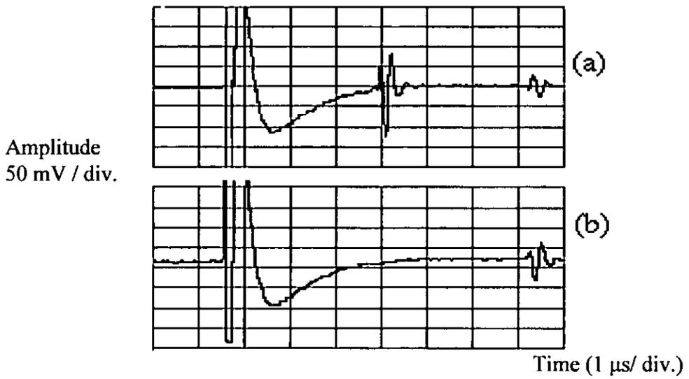
Figure 3-24 Experimental results using PZT material with  $\pm 15$  volts excitation: (a) 5 mm and (b) 10 mm of Carbon Fibre Composite
