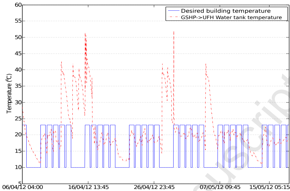
Figure 6: The recorded (hot) water temperature in the exchange vessel heated by the GSHP.
