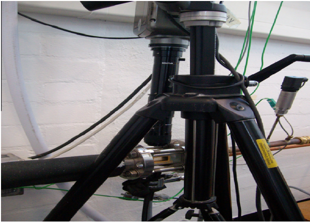
Fig. 4. Camera and sight glass set up.
