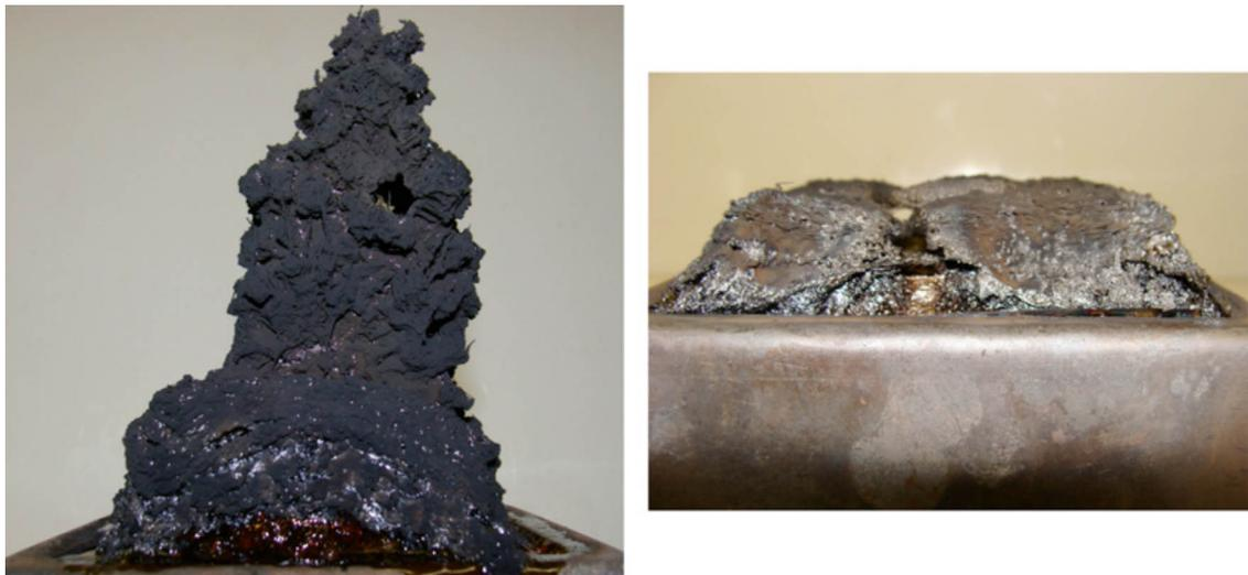
Figure 62. Six millimeter thick samples of PC (left) and PVC (right) burnt in the cone calorimeter at  $EHF_0 = 75 \text{ kW/m}^2$ . Both tests were stopped at about 200 seconds: the samples were removed from under the cone and photographed.
