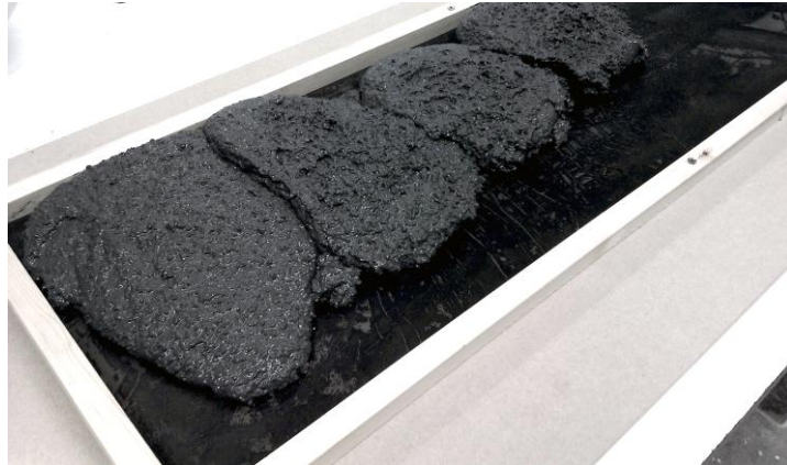
3. Casting onto print plates
