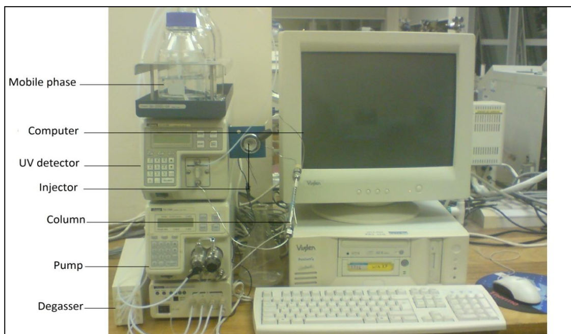
Figure 2.1 HPLC set-up used for the analysis.
