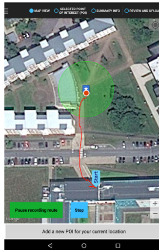
Figure 3. Illustrative Screenshot showing the presentation of a default geo-fence (in the ‘MAP VIEW’ tab) representing the trigger zone associated with a newly created POI.
