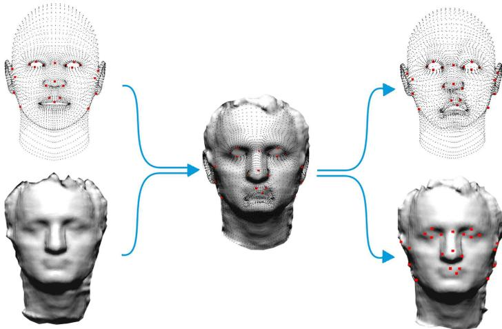
**Fig. 11** Labelling process. Inputs: Manually labelled deformable model (top left) and 3D reconstruction (bottom left). The model registered to the reconstruction (centre). Outputs: Deformed model (top right) and labels transferred from the model to the 3D reconstruction (bottom right).
