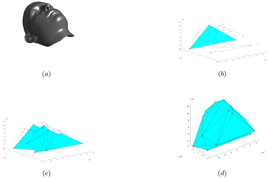
**Fig. 2** The growth of the filtered complex associated to a face mesh: (a) single vertices associated with landmark points (superimposed on a template face model); (b) some edges and the first face appear; (c) almost all the simplices appear; (d) the Delaunay complex of the face mesh.
