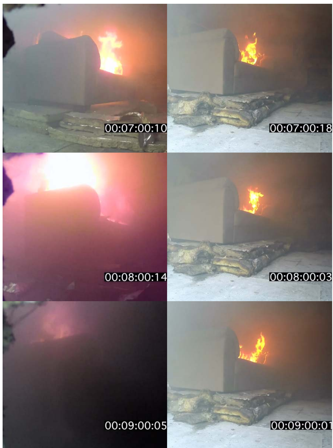
Plate 18 – Image of fire development Exp.07 and Exp.03 (7 to 9 min)
