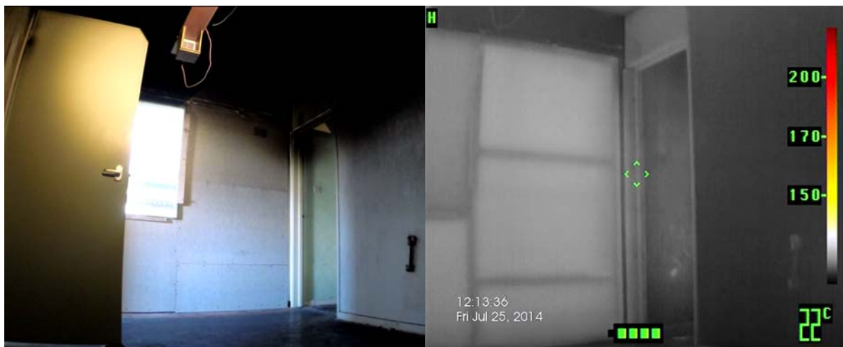
Plate 11 – Images from within the hallway for Experiment 04 (10s after ignition)
