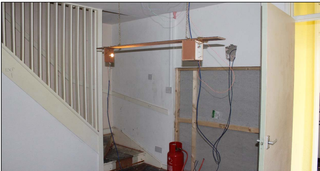
Plate 3 – Visual obscuration monitoring equipment
