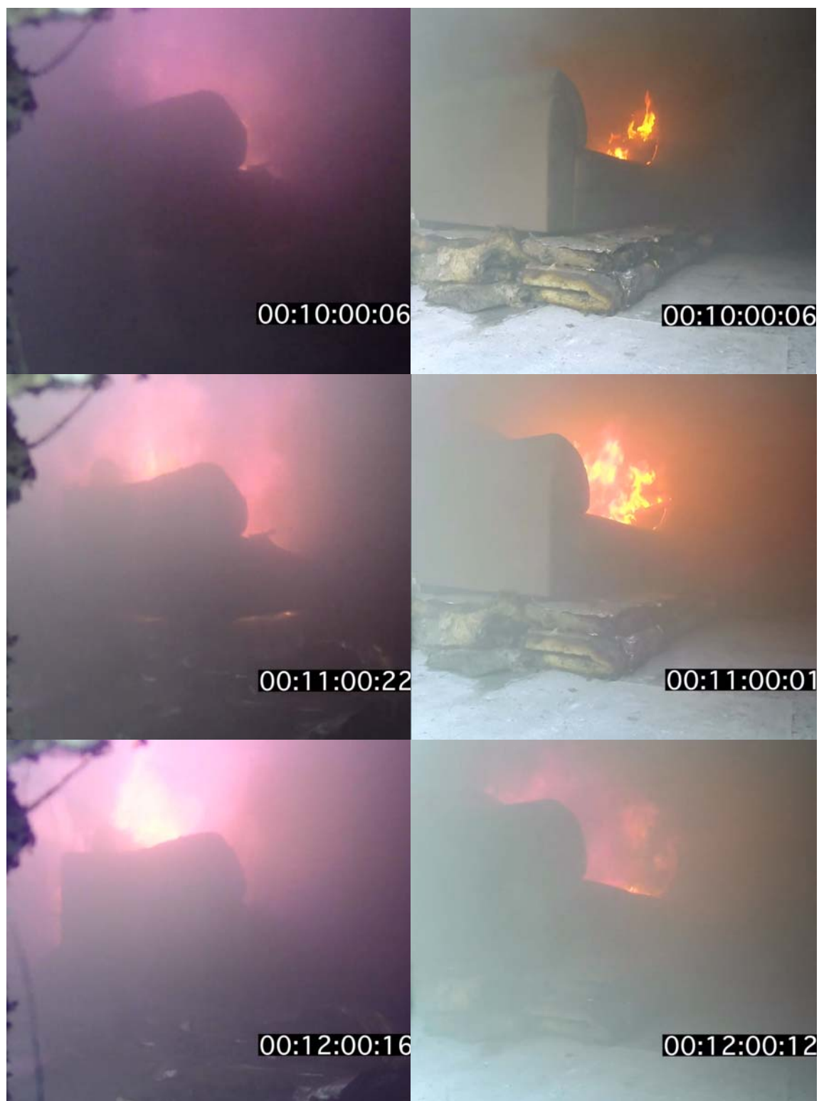
Plate 19 – Image of fire development Exp.07 and Exp.03 (10 to 12 min)
