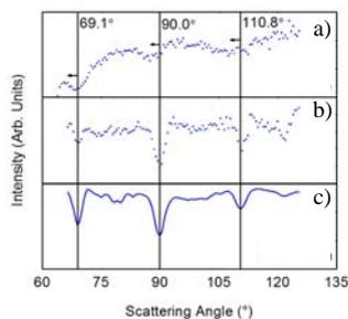
**Figure 3.** One-dimensional spectra taken along the angle axis, showing the intensity of scattered ions as a function of angle. (a) For the top-most layers (b) for the sub-surface region and (c) a simulated spectrum of the same material.
