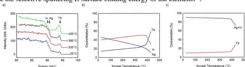
**Figure 2.** (a) 1D energy spectra from the five-fold *i*-Ag-In-Yb surface after sputtering and annealing at different temperatures. Peaks relating to Yb, Ag and In are highlighted. (b) Concentrations of Yb, Ag and In in the top-most layers versus annealing temperature extracted from (a) by fitting with the SIMNRA simulation program. (c) Concentrations of Yb and Ag + In combined for the sub-surface region
