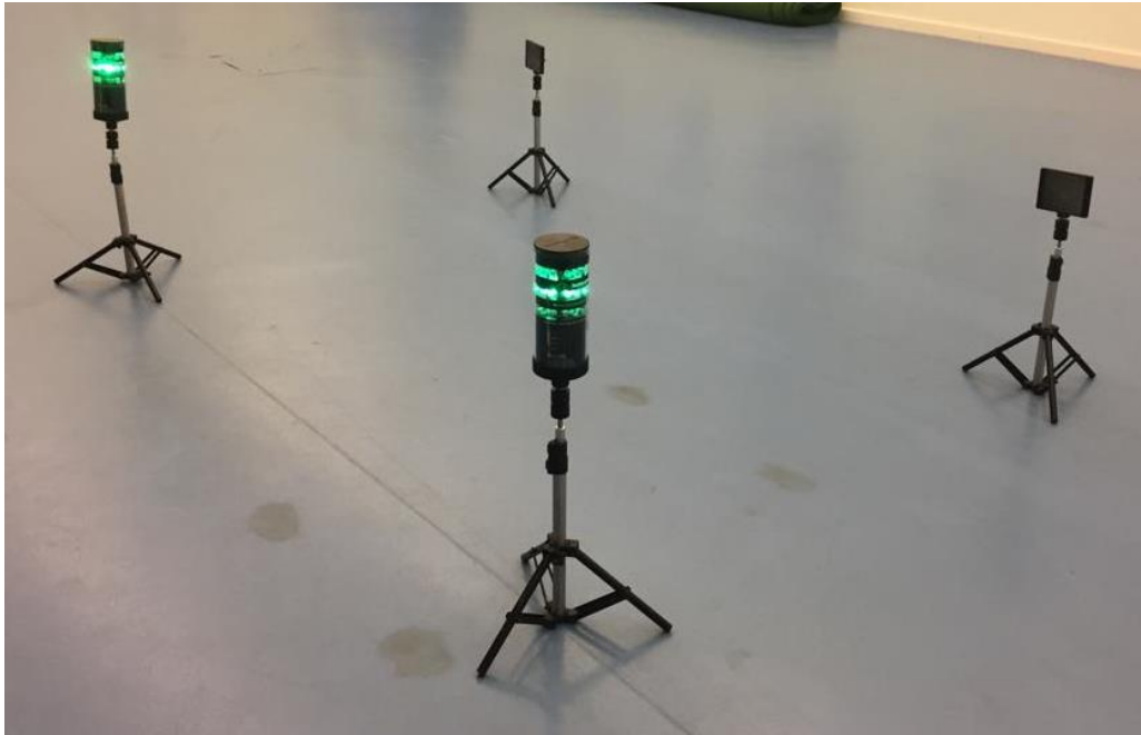
Figure 3.8: Examples of the SmartSpeed timing gate system (reflectors and emitters).
