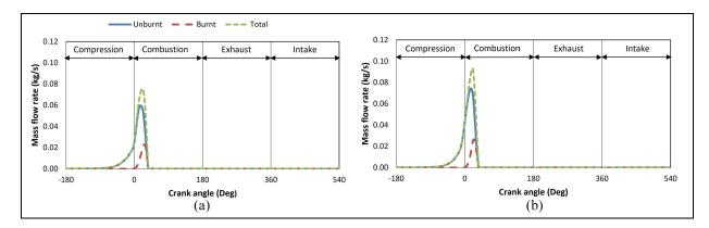
**Figure 10.** Total burnt and unburnt gas leakage from the combustion chamber into the piston ring-pack top crevice volume in an engine with: (a) CDA, and (b) normal operation.
