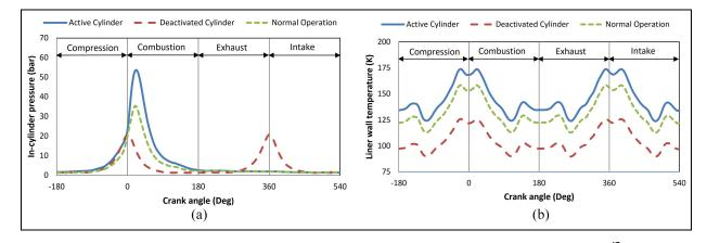
Figure 4. Measured engine data: (a) in-cylinder pressure, and (b) liner wall temperature at 3000 rpm and full load.<sup>47</sup>
