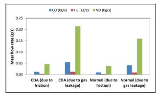
**Figure 13.** Breakdown of total emissions' flow rate due to friction and gas leakage.
