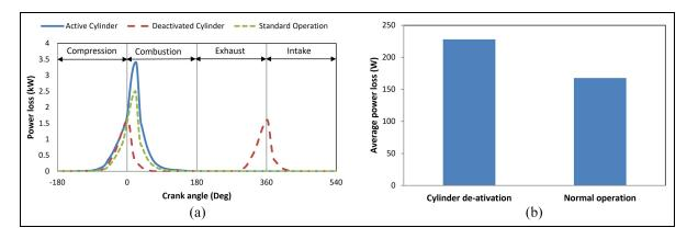
Figure 8. Gas leakage power loss predictions in an engine cycle under normal operation and cylinder deactivation: (a) per crank angle, and (b) average per cycle.
