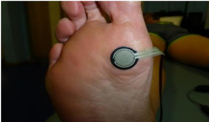
The FSR signal was checked by examining the signal trace which was completed prior to proceeding to the test trials. If the FSR signal was poor, the FSR was repositioned and the process was repeated until the signal trace was acceptable. This was deemed to be when there were clear increases in force coinciding with the participant putting pressure on the head of their first metatarsal.
