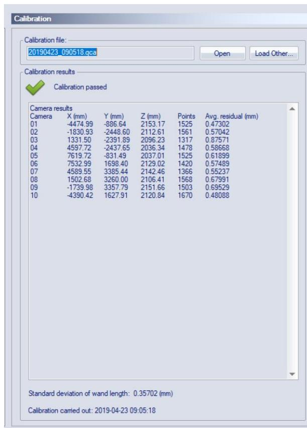
Figure 3-5 Example of the average residual errors of a successful calibration.
