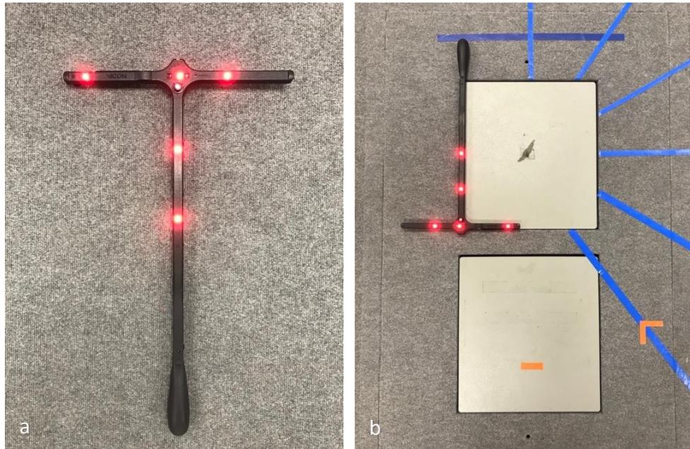
**Figure 3-10 a) Active Calibration Wand,
