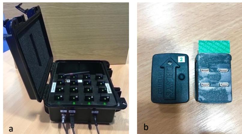
**Figure 3-13 The Delsys Trigno System a) The Delsys Trigno System Base, b) The Delsys Trigno EMG sensor.**
