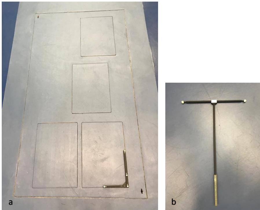
Figure 3-4 a) L-shaped reference frame on force platform 1,
