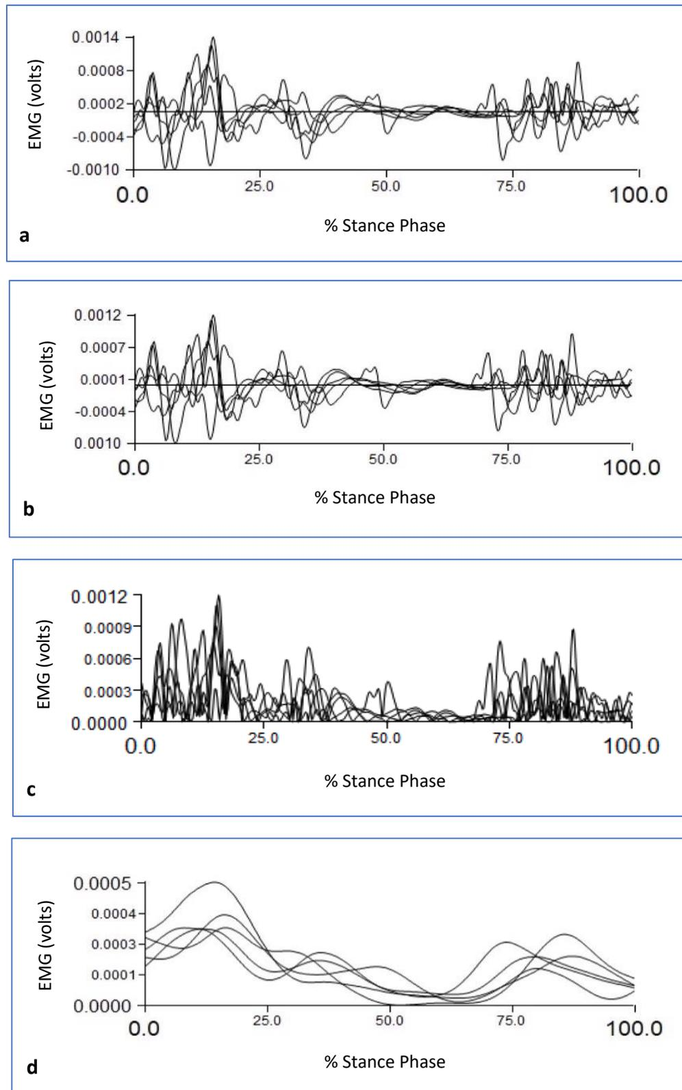
**Figure 3-36** An example of the EMG signal processing steps; a) Raw sEMG signal, b) High-pass filtered sEMG signal at 20 Hz, c) Full wave rectified sEMG signal, d) Full wave rectified and enveloped using a 15Hz low pass filter.
