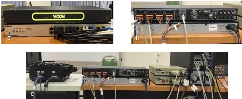
**Figure 3-12 Synchronisation of the Vicon Vantage, AMTI force platforms and Delsys systems a) Vicon lock box (front), b) Vicon lock box (back), c) Complete integration and synchronisation of equipment.**
