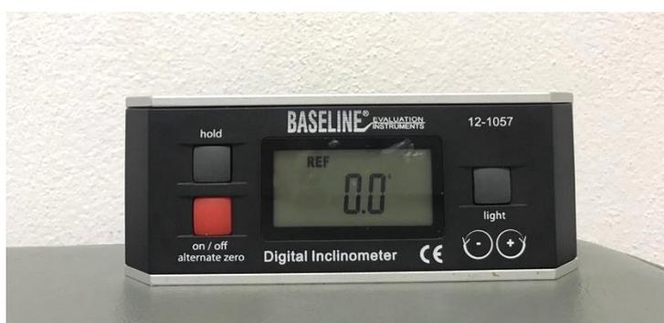
**Figure 6-5 Baseline® Digital Inclinometer.**
