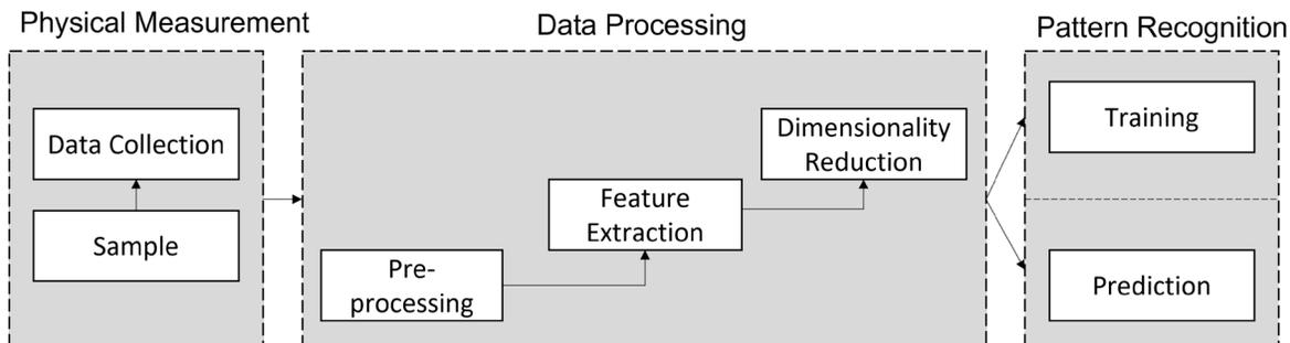
Figure 2. A diagram of the e-nose workflow.
