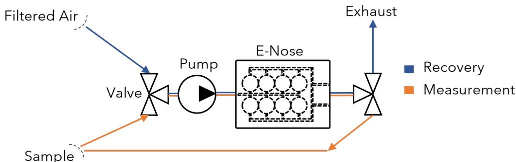
Figure 3. A schematic diagram of the experimental setup. There are two paths for gas to flow: filtered air is used during recovery and is immediately exhausted, sample air is recirculated between the sensor headspace and then back into the sample headspace. Note that the e-nose has eight but only six sensors are used.
