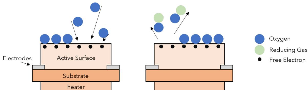
Figure 1. Function of a MOS gas sensor. As oxygen binds to the active surface its resistance increases; this resistance then decreases as reducing gases out-compete the binding sites.
