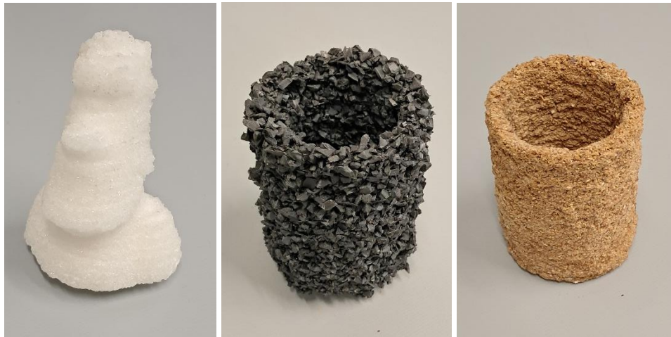
Figure 15. Left: Sugar/Sugar syrup moai. Middle: Granulated polystyrene waste/ABS-acetone cup. Right: Sawdust/Epoxy cup. Source: Authors own work.
