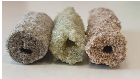
Figure 11. Hollow tubes were consistently formed in large single tracks bound with sodium silicate. Source: Authors own work.
