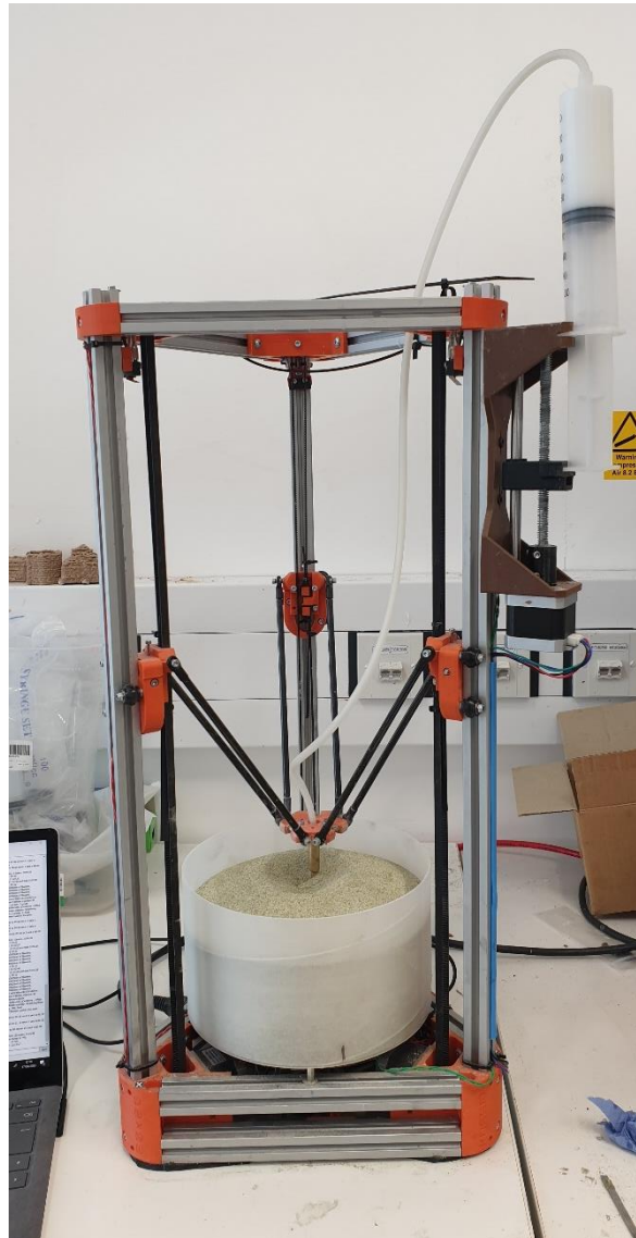
Figure 2. Modified delta 3D printer for binder injection AM. Source: Authors own work.
