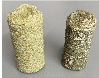
Figure 17. Glass samples. Left: As printed. Right: Reduced size after sintering. Source: Authors own work.
