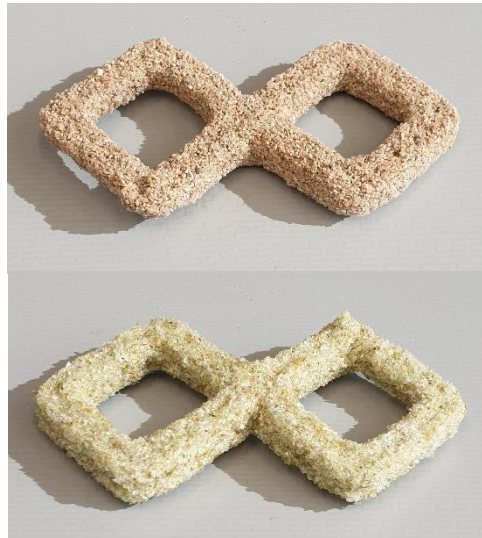
Figure 12. Custom diamond toolpath designed to test self-intersection of the toolpath printed with sand/PVA and glass/PVA. Source: Authors own work.
