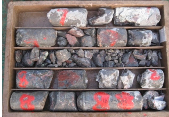
Fig. 2. M1Z3-TWG-68 rock core obtained from a depth of (a) 8.5–12 m, and (b) 12–16.5 m.
