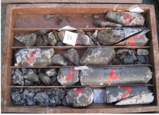
Fig. 2. M1Z3-TWG-68 rock core obtained from a depth of (a) 8.5–12 m, and (b) 12–16.5 m.
