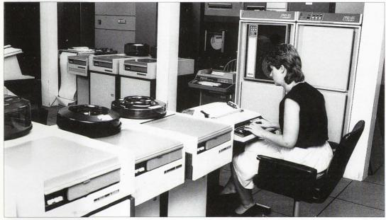
Computing Centre machine room c.1984. An operator working at a teletype terminal in front of a PRIME 750 minicomputer (one of an eventual 7) and its reel to reel tape back up unit.
