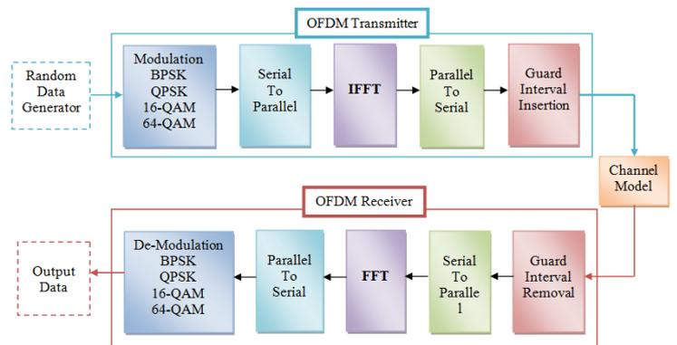
**Figure 1.** OFDM Block diagram
