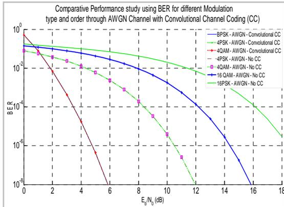
**Figure 3.** Comparative performance study using BER for PSK and QAM with/without convolutional channel coding
