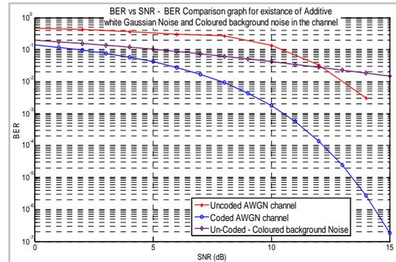
**Figure 6.** BER comparison graph for different channel scenarios, Un-coded AWGN, convolutionally coded AWGN and Channel affected by the modelled coloured background noise.
