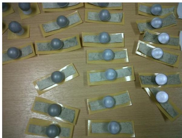
Figure 25. Reflective markers and application method used during data collection.
