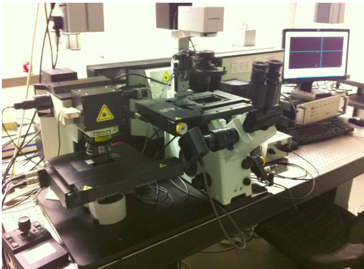
Figure 6: Horiba Jobin-Yvon LabRAM HR800 Raman spectrometer.
